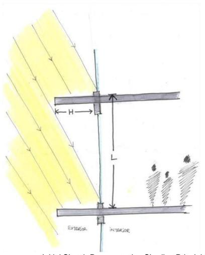
Initial Sketch Demonstrating Shading Principle
