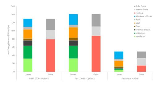
Figure 1 - Results of Etude PHPP modelling for a typical semi-detached dwelling: Space heat demand must be lower to deliver net zero carbon homes.
