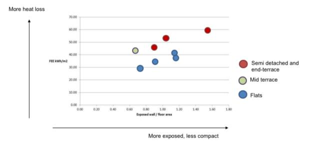
On the contrary, an unintended consequence of the notional building approach is that a building with a shape leading to HIGHER total heat loss can perform better against Part L
