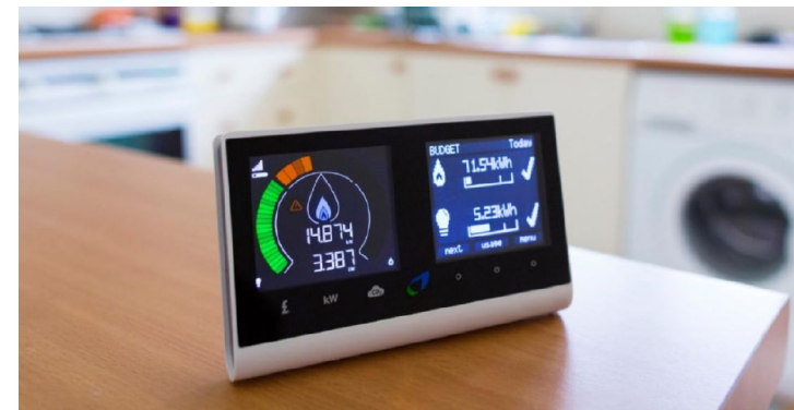
Energy display monitor: users should be able to compare predicted energy use from SAP/RdSAP with the readings from energy meters, display monitors or bills.
