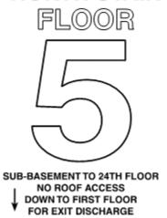
Figure A.7.2.2.5.4 Example of a Stairway Marking Sign.
