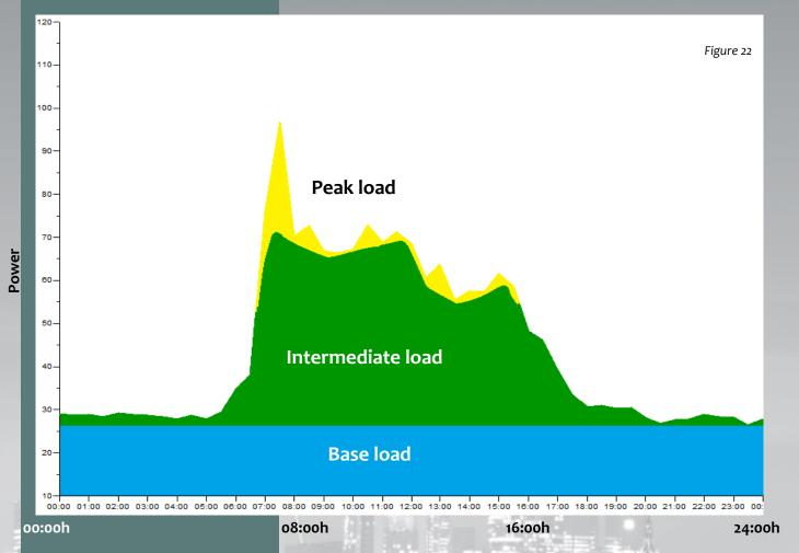
Base load is the minimum amount of power over a given period, that is, the basic amount of electricity that is always required on a 24/7 basis.
