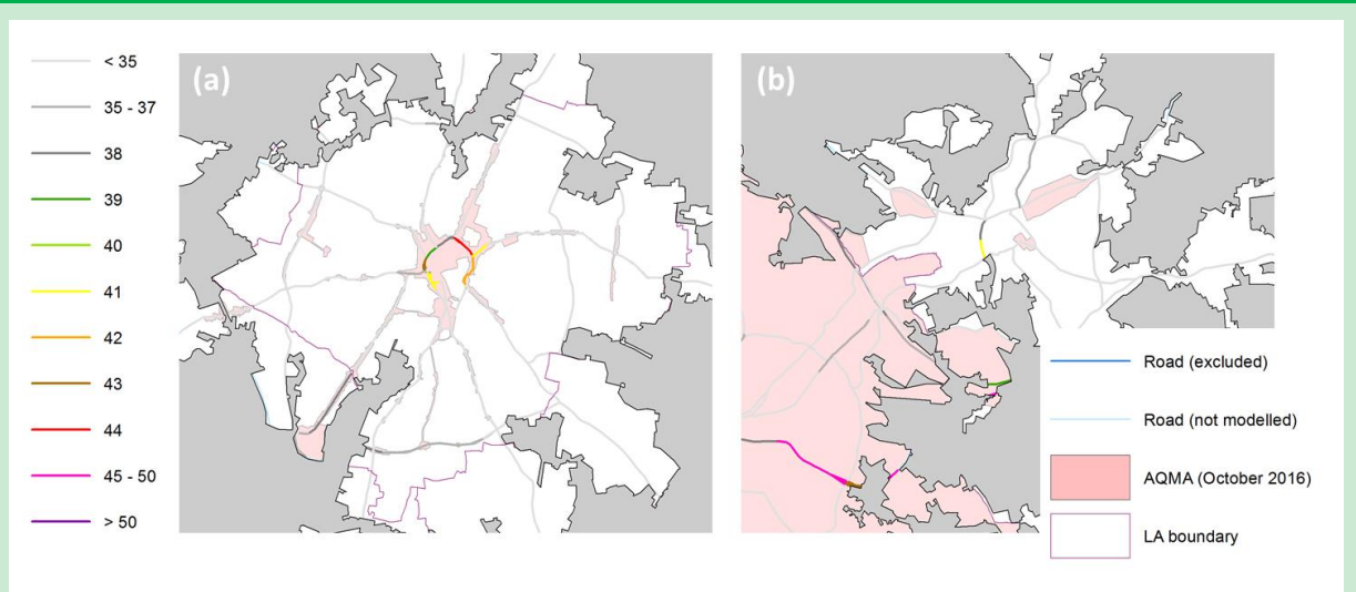
Figure 2.6: Examples of orientation of roadside exceedances; showing exceedances contained within an urban centre (a), and exceedances located on routes into the city and on a bypass (b)
