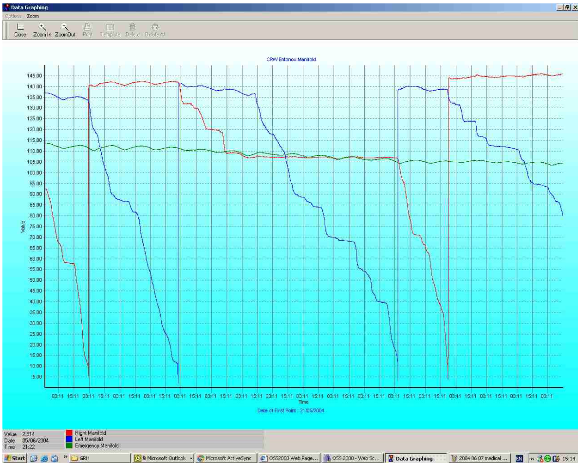
Figure 28: shows pressure decay in manifolds as gas is consumed.
