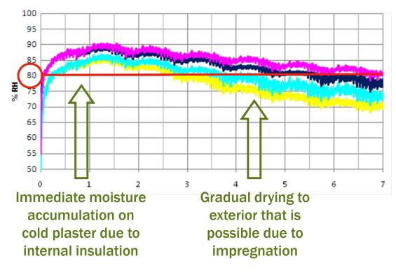
Mineral wool internal insulation on solid brick substrate
