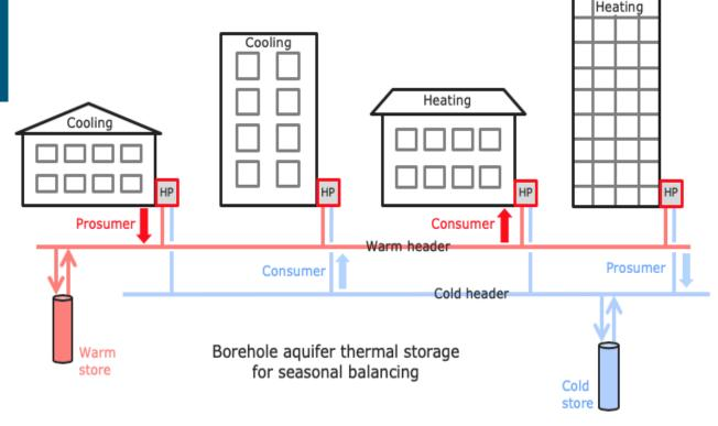
5DHC is a good solution where there is a significant mix of cooling and heating demands, allowing prosuming across the heat network itself
